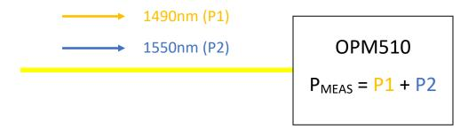
As you can see the technician would never be able to tell if the data signal was present or not since it is so much smaller than the video overlay signal.
