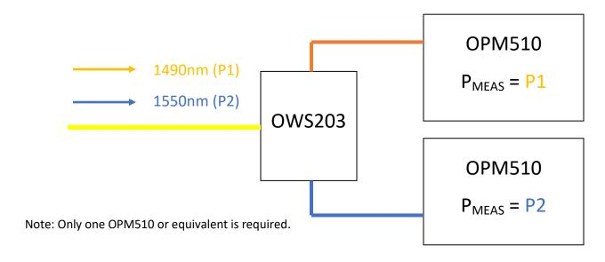
P1 would be measured at -17dBm and P2 would be measured to be 0dBm. The technician can now measure each signal with certainty and no influence from the adjacent wavelength.
