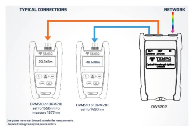
The loss of the OWS200 has negligible effect on the measurements as the OWS loss is typically less than 0.1dB. In the above example the OPM used to measure 1577nm is set to 1550nm. Errors due to not measuring at the exact wavelength are small since the responsivity of an InGaAs OPM is very flat over the 1530 - 1625nm range.
