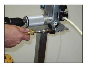
7. Attach air supply hose (from air compressor or nitrogen bottle) to the ULTIMAZ.
