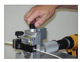
6. With the cable installed through the cartridge and into the duct, turn the tension control knob fully clockwise until snug.
