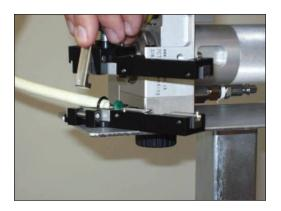
2. Insert the duct end in the inserts with the O-ring in the groove, while putting the two black cartridge insert halves back together by aligning the guide pin. Align the cartridge halves and press them together. Make sure the duct and O-ring and cable seal stay seated in the insert during the process. Once properly aligned and together with the duct fully seated, snap the cartridge locking clips into place.
