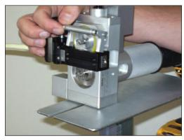
4. Place cartridge into the unit being sure it is positioned properly. Pull down the locking bar to secure the cartridge in the receptacle. The tension control knob should be in the counterclockwise position. The compression knob (on the cartridge) should be on the operator's right when in the installation position. Cables are always installed from the operators left to right.
