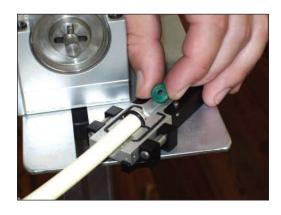
1. Holding the black duct/cable insert "cartridge" halves in one hand, or laying on a level surface such as the ULTIMAZ Operators Stand, install the silver duct/cable inserts into each half. The insert with the rubber sealing cord is ALWAYS on the bottom and is placed in the cartridge half without the compression knob. Place the proper size cable seal in the insert. The "grooved side" should be facing back into the cartridge. Next, place the correct size O-ring on the microduct end.
