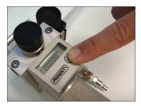
8. Re-Set counter to zero by depressing re-set button and holding until display clears.
