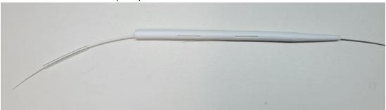
2. Cleave the field and splice on connector fibers and load into the fusion splicer.
