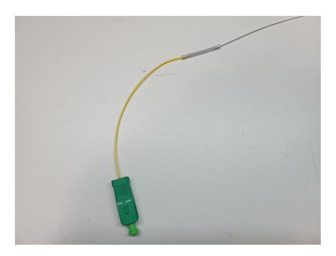
6. Place the strain relief boot onto the splice on connector.
