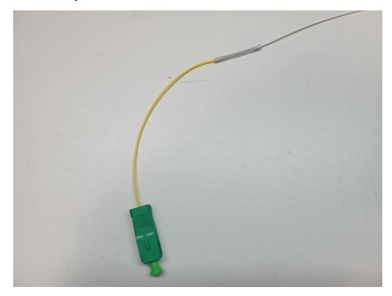
5. Shrink the splice protector and allow to cool in the cooling tray.
