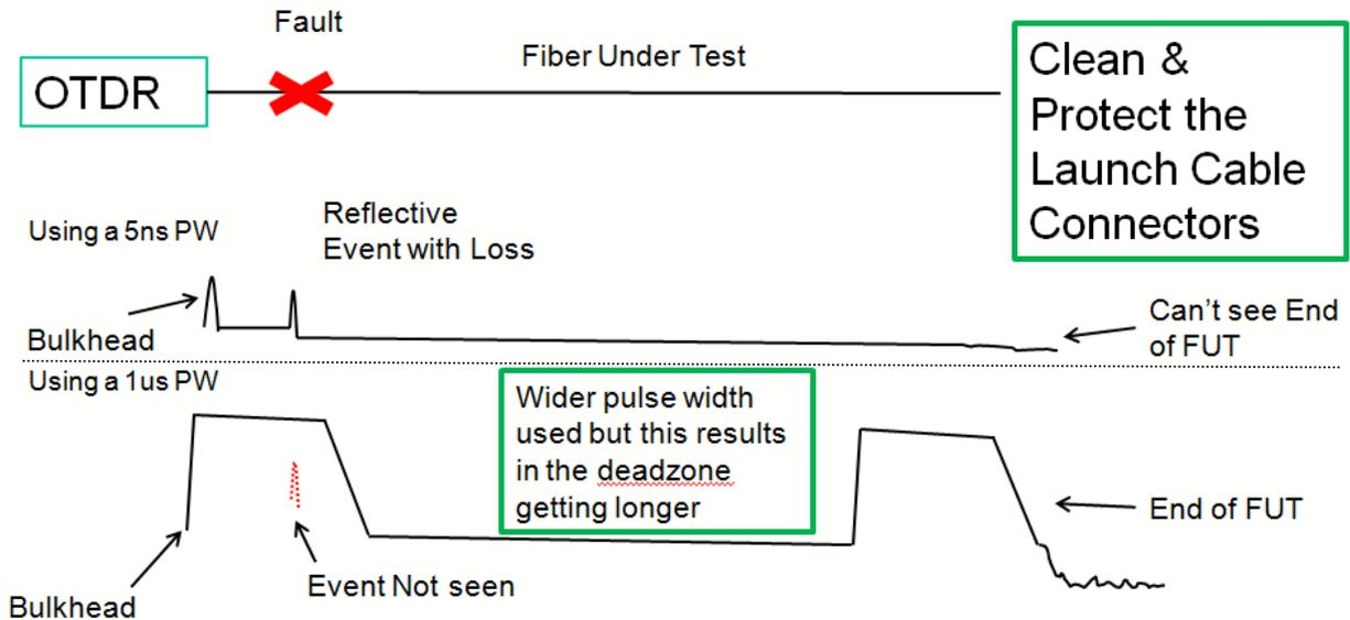
Here you can see that with a 5ns pulse width the fault can be easily measured but the end of the fiber can't be seen. If a wider pulse width is used (1us) the fault can no longer be measured. This is because the event deadzone has become too long and the bulkhead and fault are now represented as one pulse.
